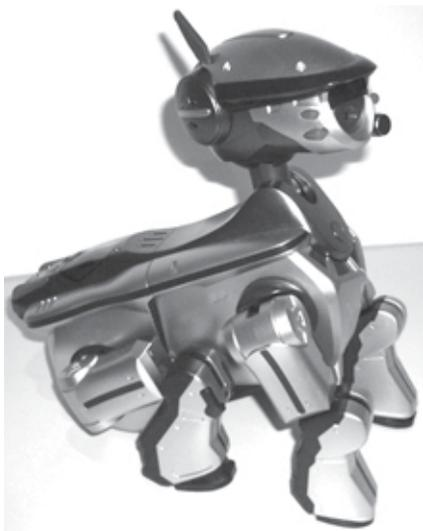
*The futuristic ERS-220 AIBO. Available in silver only, the ERS-220 has the most robotic look of all AIBO models. It has a headlight in the middle of its head, an antenna instead of an ear, many colorful lights, and a more tonal sound than the ERS-210 model. There is also an ERS-220A, which, like the ERS-210A, has a faster processor.*
